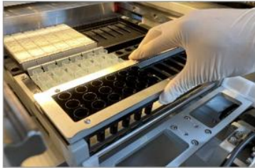
Put Holder Lid on (arrows facing to the inside)
